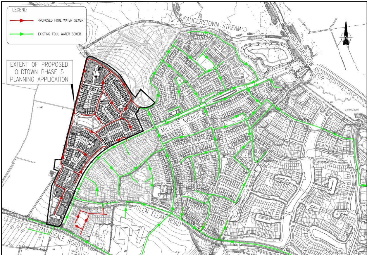
Figure 3 | Existing and Proposed Foul Water Drainage
