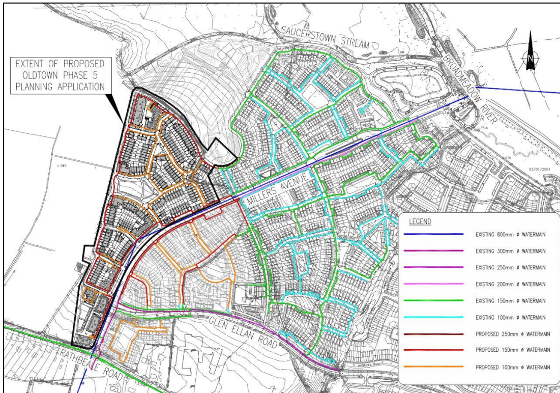
Figure 6 | Existing and Proposed Water Supply Network
